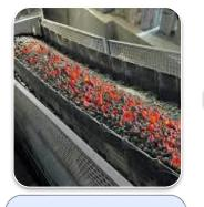
Hot clinker exits from kiln and enters the clinker cooler to reduce its temperature from 1450 °C to 100 °C.
