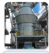
Cooled clinker mixed with gypsum and other additions. It is grinded into fine and homogenous powder, cement.
