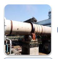
Raw meal is heated at a temperature of ~1,450 °C in a cement kiln to produce clinker.
