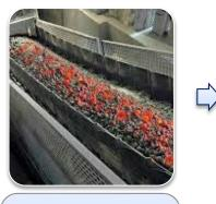
Hot clinker exits from kiln and enters the clinker cooler to reduce its temperature from 1450 °C to 100 °C.
