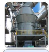
Cooled clinker mixed with gypsum and other additions. It is grinded into fine and homogenous powder, cement.
